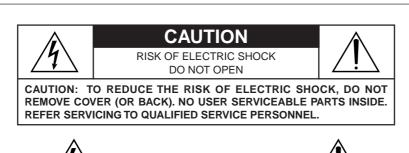
The lightning flash with the arrowhead symbol within an equilateral triangle, is intended to alert the user to the presence of uninsulated "dangerous voltage" within the product's enclosure that may be of sufficient magnitude
